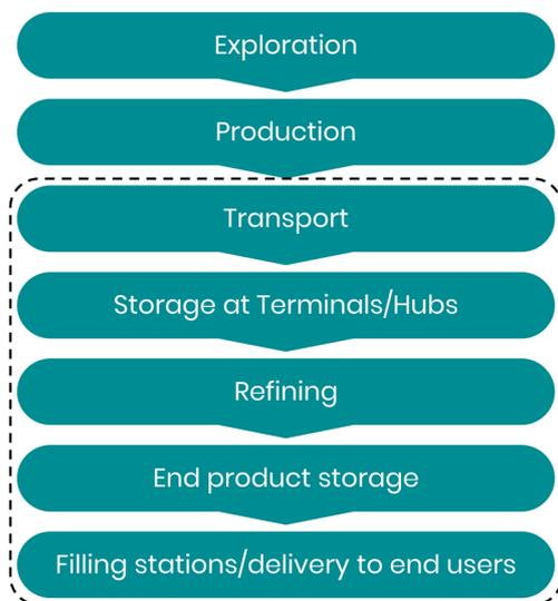
**Figure 13: Simplified representation of the oil and gas-industry value chain. Relevant steps for powerfuels are highlighted in the black box.**
