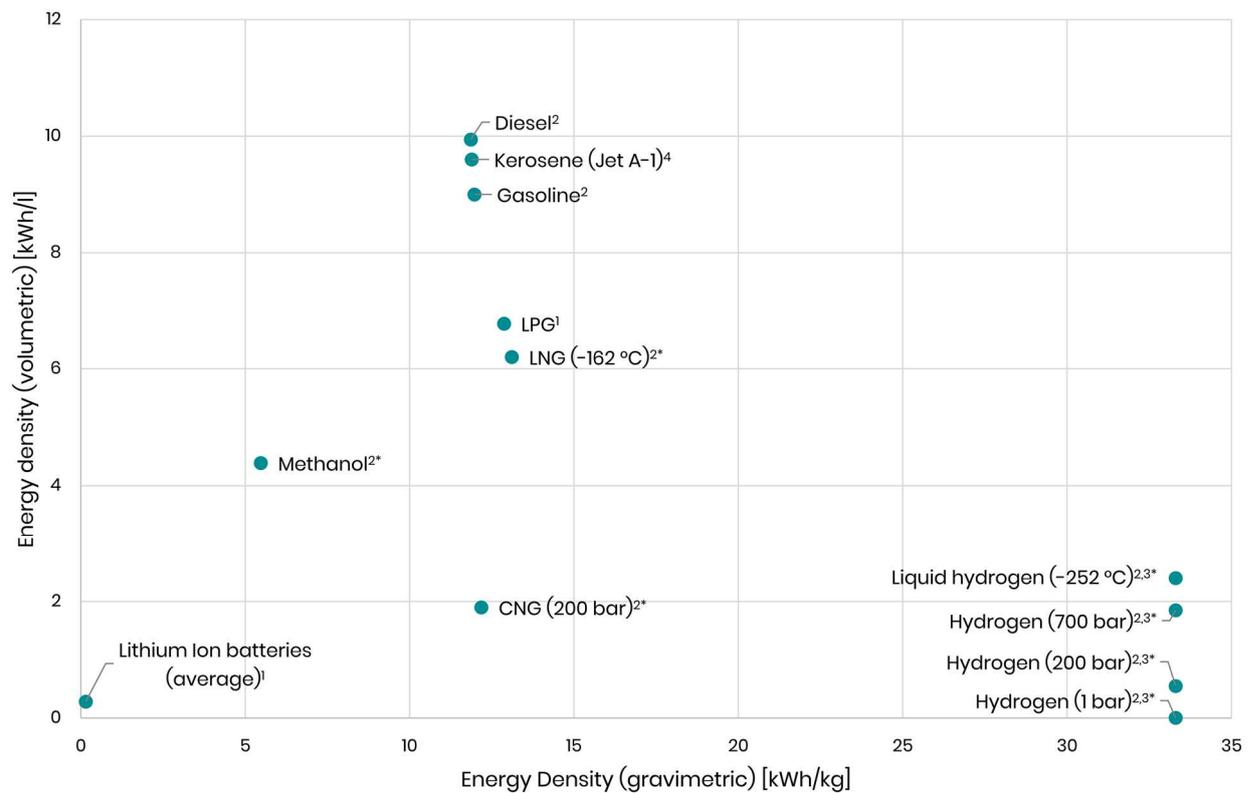
Figure 3: The gravimetric and volumetric energy density of various energy carriers (\* based on LHV)<sup>2</sup>
