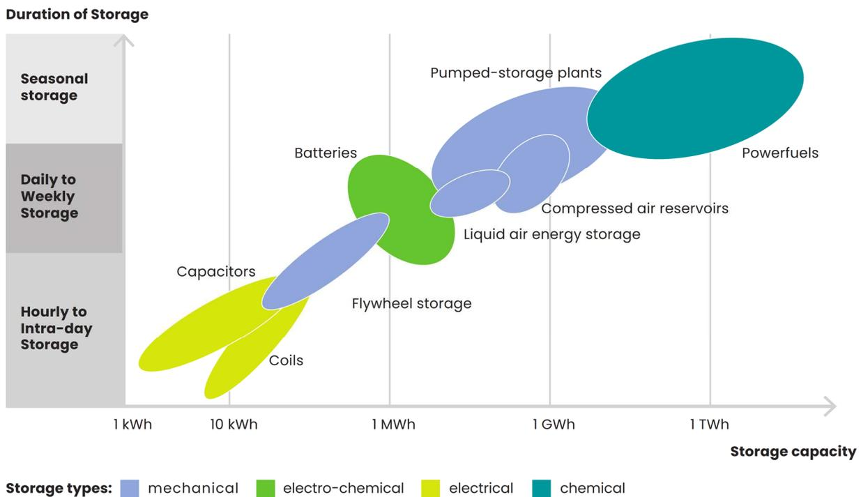
Figure 12: Common energy storage options compared with respect to storage capacity and the duration of storage (Based on Sterner and Stadler, 2014; Perner and Bothe, 2018)
