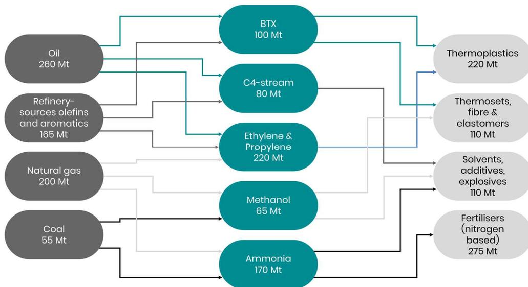
**Figure 11** Simplified scheme of fossil resources and product flows in the chemical industry in 2013 (BTX: benzene, toluene, xylene) (Based on data from (IEA, 2018b; Levi and Cullen, 2018))
